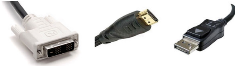
Fig. 5.8 Connectors of different digital display interfaces. From left to right: DVI, HDMI, DisplayPort
